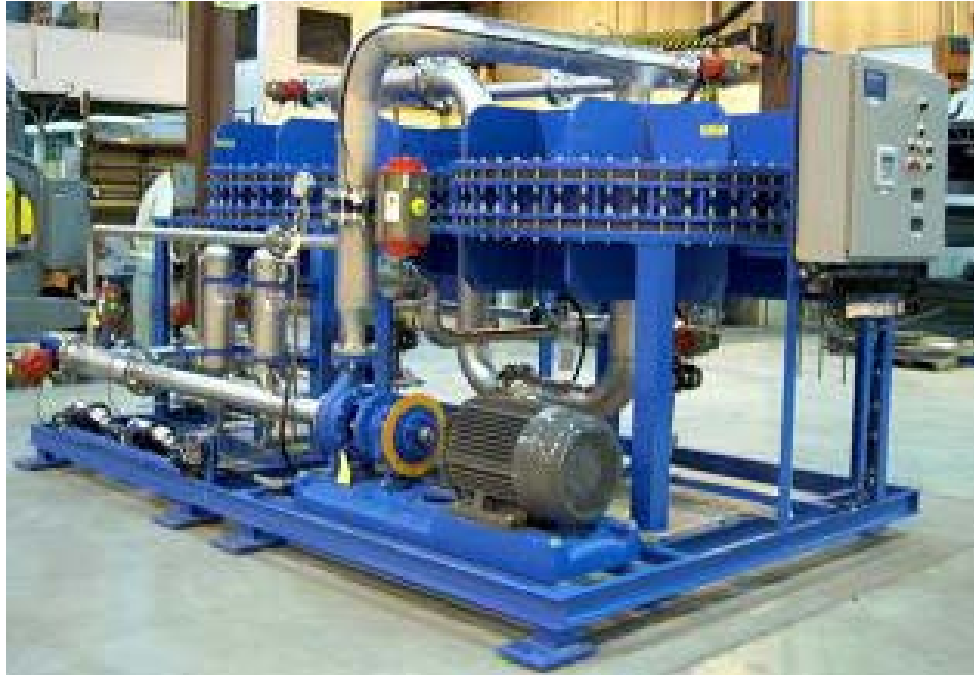
Figure F-6. Picture of a compressed bed ion exchange unit.
